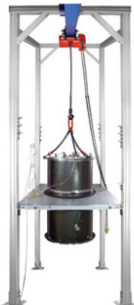
Prototype of the new hot-air engine under development in Eric Cornell’s lab at JILA. The engine is being designed to capture waste heat from refineries and other industrial plants to make electricity.
