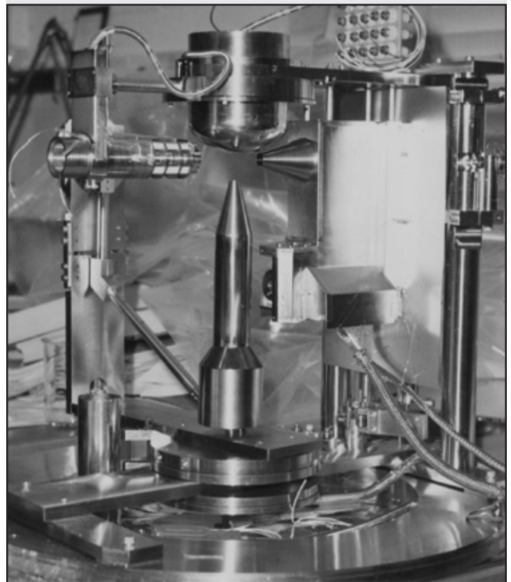
Electron impact ionization apparatus. A gas jet directed downward from the dome in the center crosses an electron beam from the electron gun at the left. Scattered incident electrons and electrons knocked-out of the target atoms are detected by the electron analyzer at the right and by the moveable analyzer that is positioned below the scattering center. Credit: JILA
