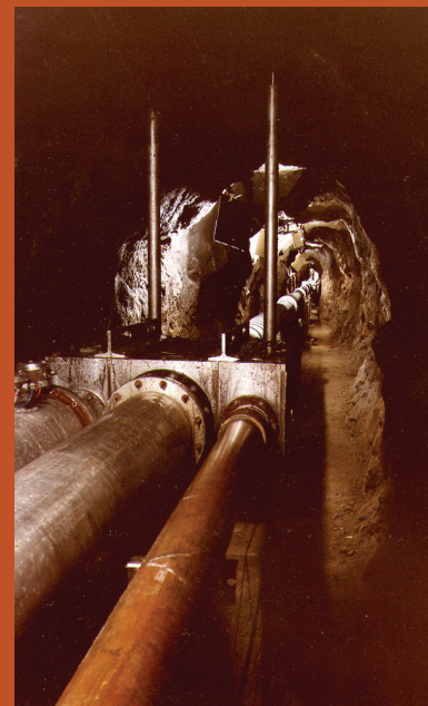
The 30-m interferometer inside the Poorman mine. Credit: JILA
